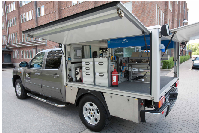
Figure 3.1: The mobile gamma-ray spectrometry vehicle of the SSM, used in Paper IV. The blue boxes suspended in the roof are the two NaI(Tl)-detectors, whereas the HPGe (beige-coloured cryostat) can be seen in the centre of the rear compartment. Image courtesy of Bosse Alenius, SSM.
