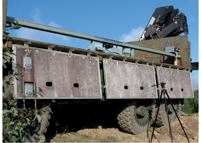
Figure 2. The linear positioner mounted on the bed of the truck. The horn antennas, shown in the far end of the rail, are connected with phase-stabilized cables to the PNA network analyzer.
