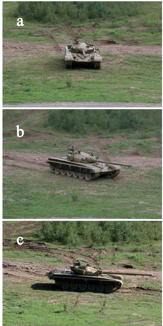
Figure 5. Photographs of the T72 tank at three different angles. The aspect angles are a) 0^\circ , b) 45^\circ c) and 90^\circ .
