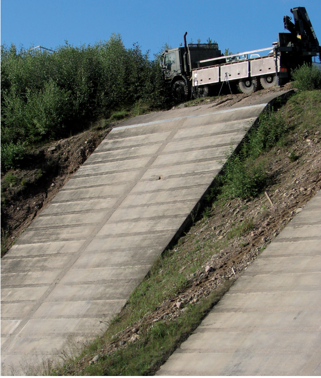
Figure 1. The figure shows the SAR setup. The linear positioner can be seen mounted on the bed of the truck. The elevation gives a SAR look angle of 10^\circ .
