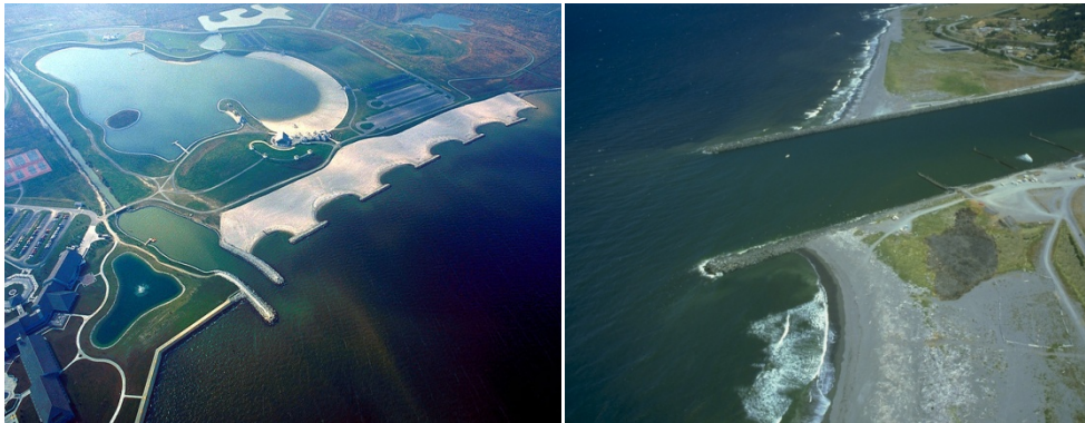
Fig. 1a. Tombolo formation behind the detached breakwaters at Maumee Bay State Park, Ohio, USA (Ken Winters, U.S. Army Corp. Eng., 1992)
