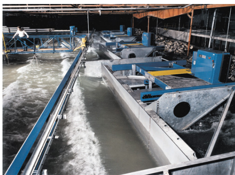
Fig. 5a. Wave-maker layout in LSTF basin (from CHL official website)
