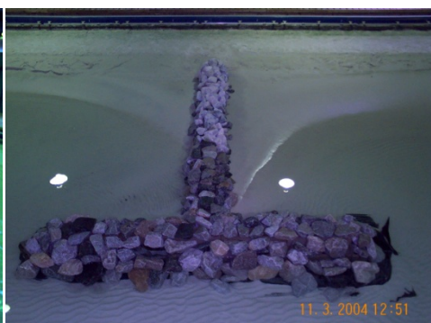
Fig. 8b. Salient developed after T3C4 (from Gravens and Wang, 2004)
