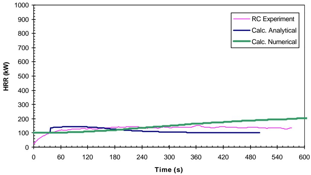
**Figure F.6:** Material M6 (FR Chipboard) HRR Comparison – RC Test Scenario
