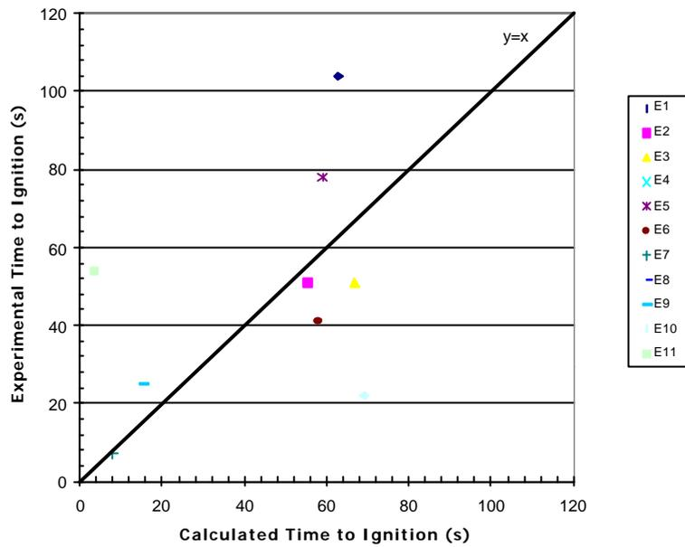
**Figure 4.3:** Time to Ignition @35kWm<sup>-2</sup> Comparison
