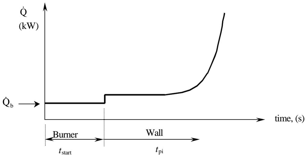
**Figure 5.2:** Characteristic Representation of the Different Ignition Times
