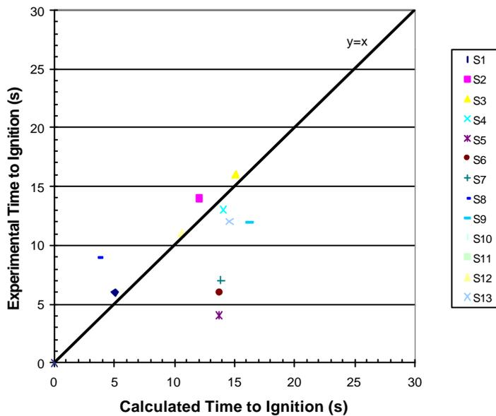
**Figure 4.4:** Time to Ignition @75kWm<sup>-2</sup> Comparison
