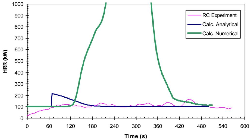
**Figure F.2:** Material M2 (FR PVC) HRR Comparison – RC Test Scenario
