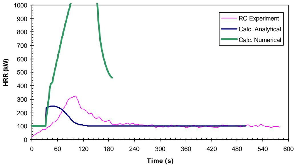
**Figure D.7:** Material S7 (Textile covering on S4) HRR Comparison – RC Test Scenario
