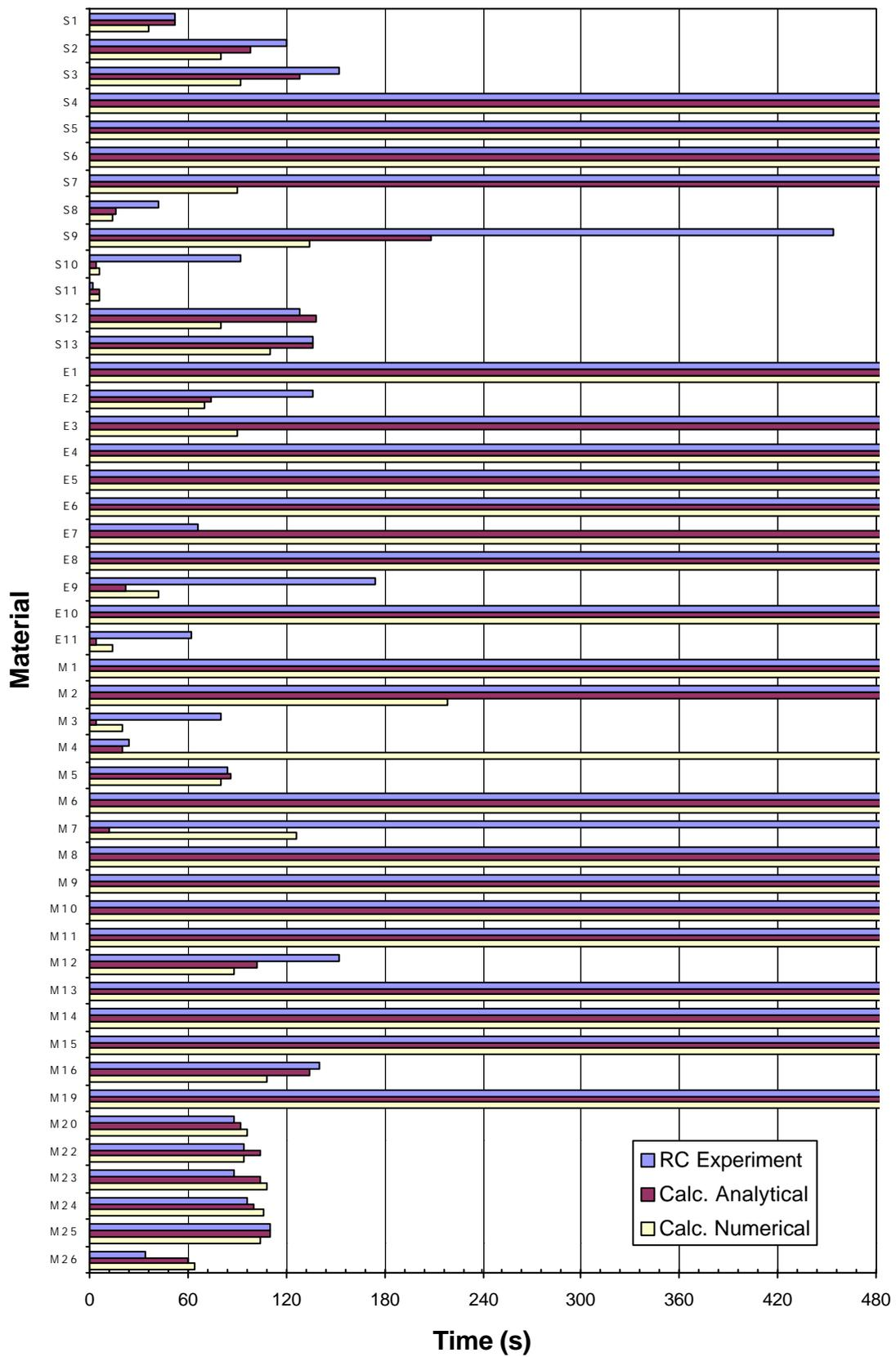
**Figure 7.2:** Room/Corner Scenario Time to Flashover Comparison
