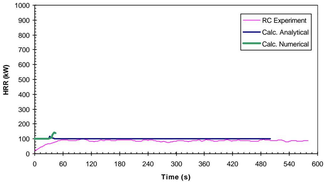
**Figure E.5:** Material E5 (Plastic faced Steel sheet on Mineral Wool) HRR Comparison – RC Test Scenario
