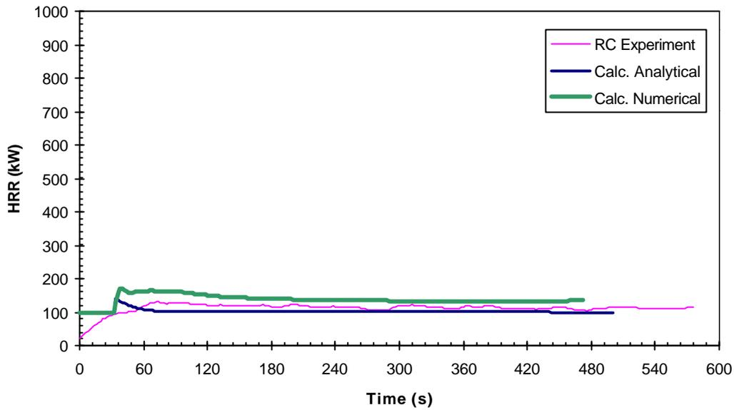
**Figure F.1:** Material M1 (Plasterboard) HRR Comparison – RC Test Scenario
