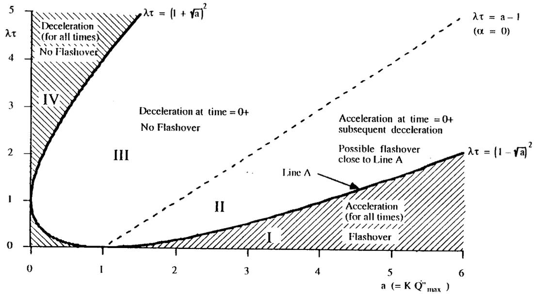
**Figure 2.5:** Regions of Flame Front Acceleration and Deceleration [17]
