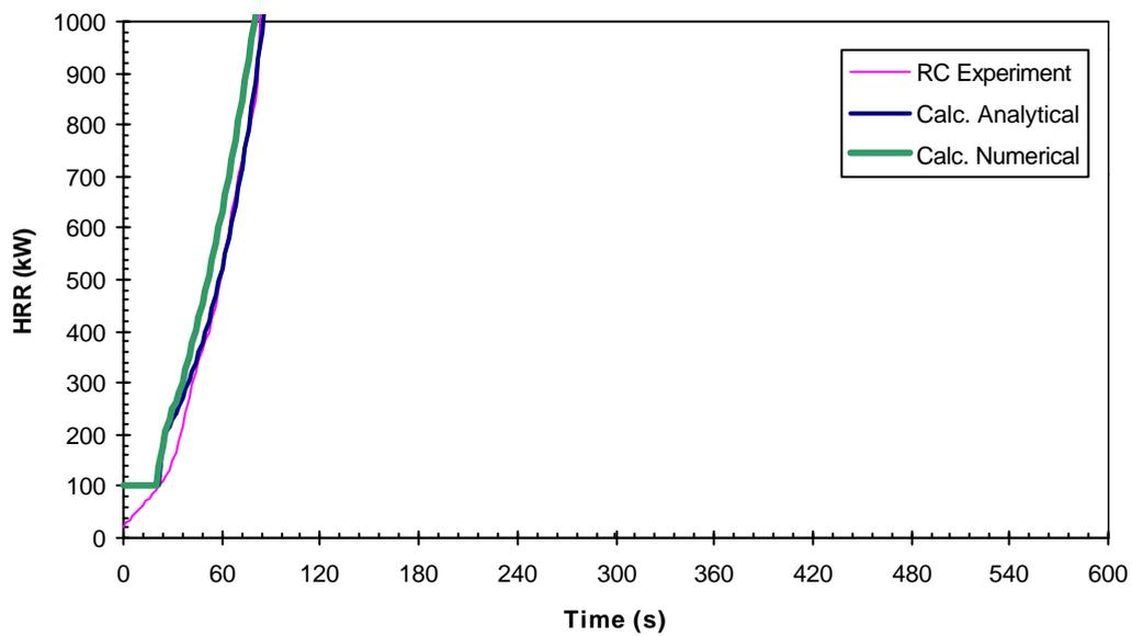
**Figure F.5:** Material M5 (varnished mass Timber, Pine) HRR Comparison – RC Test Scenario
