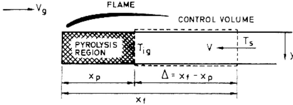
**Figure 2.1:** Energy Conservation Analysis in Wind-aided Flame Spread [17]
