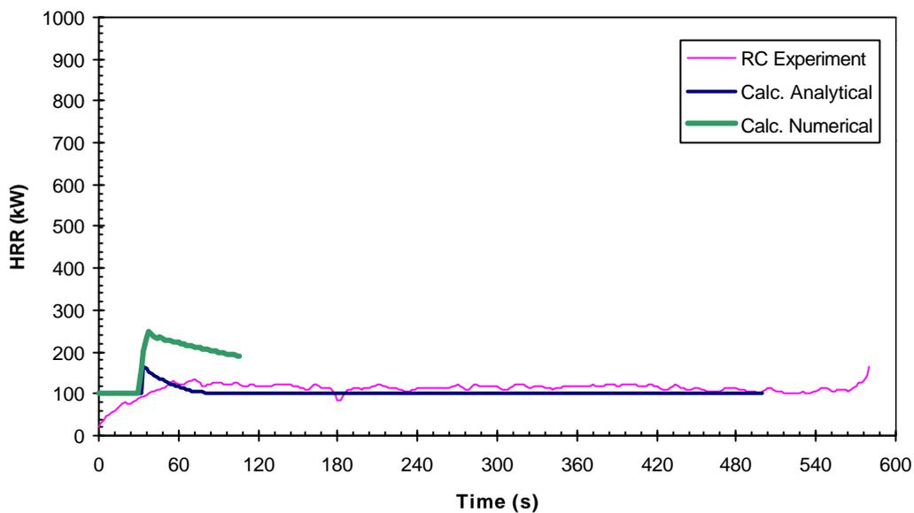
**Figure E.1** Material E1 (painted Gypsum Paper Plaster board) HRR Comparison – RC Test Scenario
