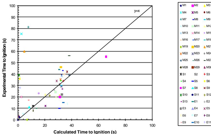
**Figure 4.2:** Time to Ignition @ $50\text{kWm}^{-2}$  Comparison
