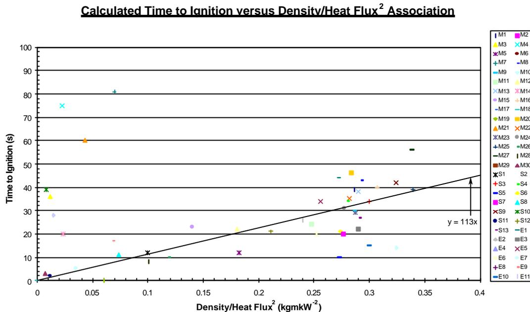
**Figure 4.1:** Time to Ignition,  $t_{ig}$ , versus  $\frac{\rho}{\dot{q}_e'^2}$  Investigation
