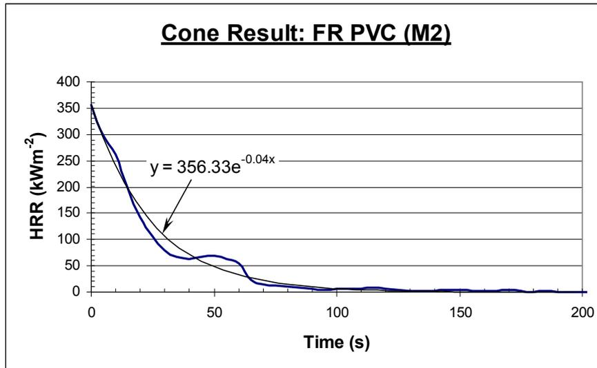
**Figure 3.5:** Typical Manipulated Cone Calorimeter Data
