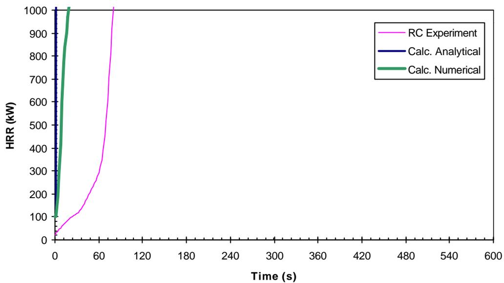
**Figure F.3:** Material M3 (FR extruded Polystyrene board) HRR Comparison – RC Test Scenario
