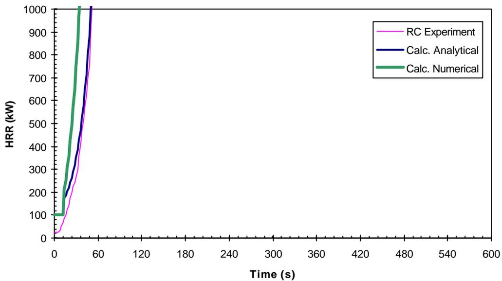
**Figure D.1:** Material S1 (insulating Fibre board) HRR Comparison – RC Test Scenario
