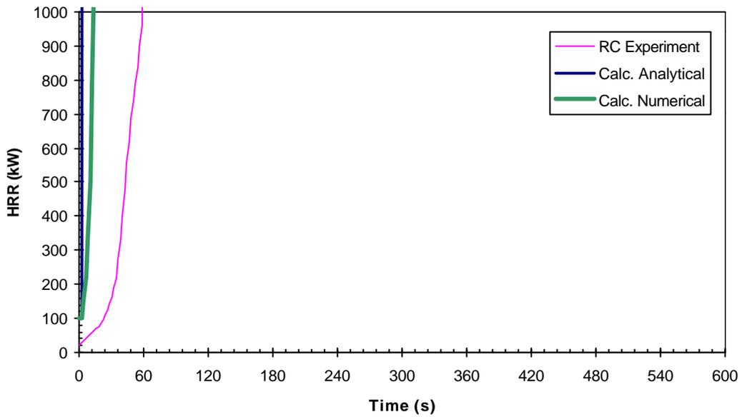
**Figure E.11:** Material E11 (FR Polystyrene) HRR Comparison – RC Test Scenario
