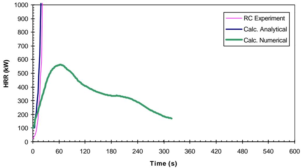
**Figure F.4:** Material M4 (PUR foam panel with Aluminium foil faces) HRR Comparison – RC Test Scenario
