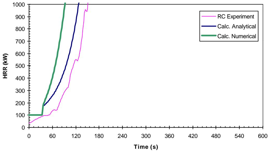
**Figure D.3:** Material S3 (Particle board) HRR Comparison – RC Test Scenario
