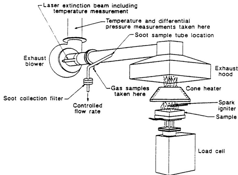
**Figure 3.1:** Typical Cone Calorimeter Experimental Set-up [17]
