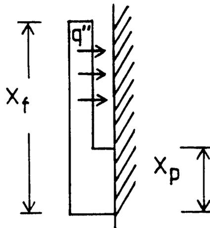
**Figure 2.2:** Constant Heat Flux Region,  $x_p < x < x_f$  [17]
