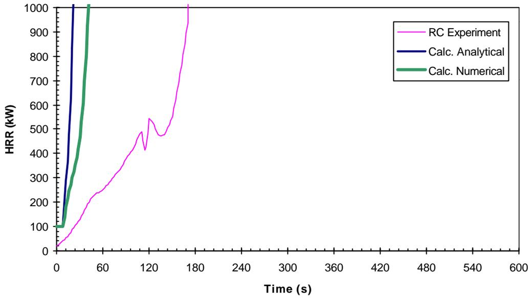
**Figure E.9:** Material E9 (Polyurethane foam covered with Steel sheet) HRR Comparison – RC Test Scenario
