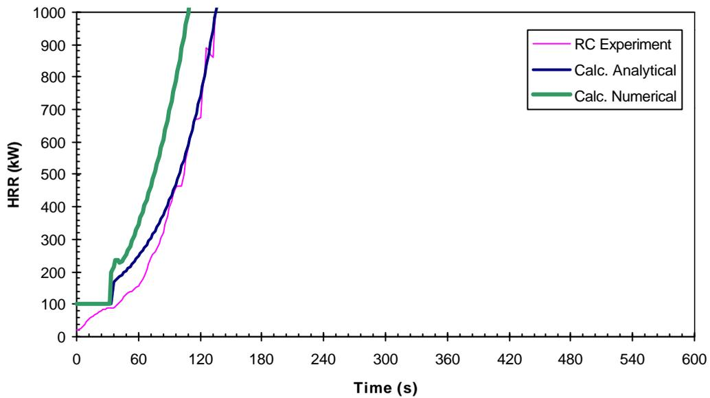
**Figure D.13:** Material S13 (Paper covering on S3) HRR Comparison – RC Test Scenario
