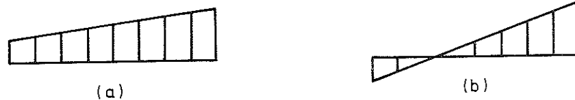
FIG. A 6. ALTERNATIVE TYPES OF STRAIN DISTRIBUTION SIMULTANEOUS WITH AN INCREASE OF AXIAL LOAD, \Delta P , ABOVE THE TANGENT MODULUS LOAD, AT THE CROSS SECTION OF THE COLUMN SUBJECTED TO MAXIMUM STRAIN: (a) WITH NO STRAIN REVERSAL; (b) WITH SOME STRAIN REVERSAL AS PREDICTED BY SHANLEY THEORY.
