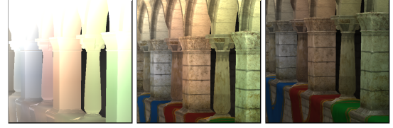
Figure 4: Samples of rendered images using the real-time implementation. The leftmost image shows only indirect illumination without any textures. The center image shows indirect illumination but with textures. The rightmost image shows the final rendering with both direct light, indirect light and textures. Note that the effect of indirect lighting has been slightly exaggerated in these images.
