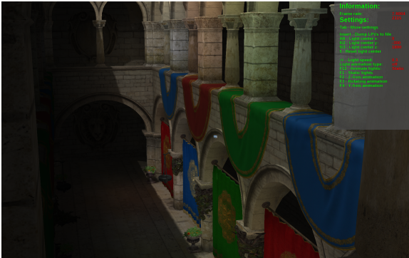
Figure 7: The final rendering of the sponza scene with both direct and indirect illumination and diffuse texturing. Note that the indirect lighting has been slightly exaggerated in this image.
