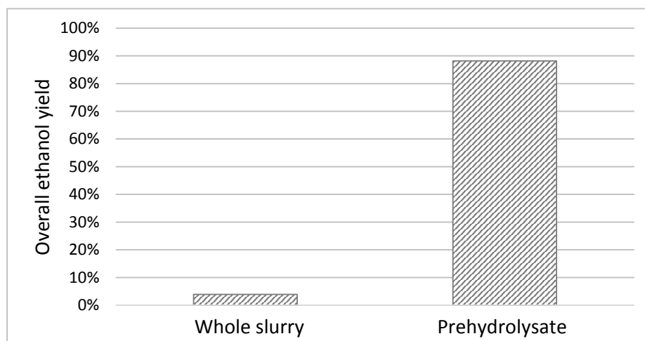
Figure 4.3: Overall ethanol yield (in % of theoretical) from SSF of steam-pretreated spruce slurry with 13.7% WIS, and SSF of prehydrolysate at a concentration corresponding to 13.7% WIS. From Paper IV.
