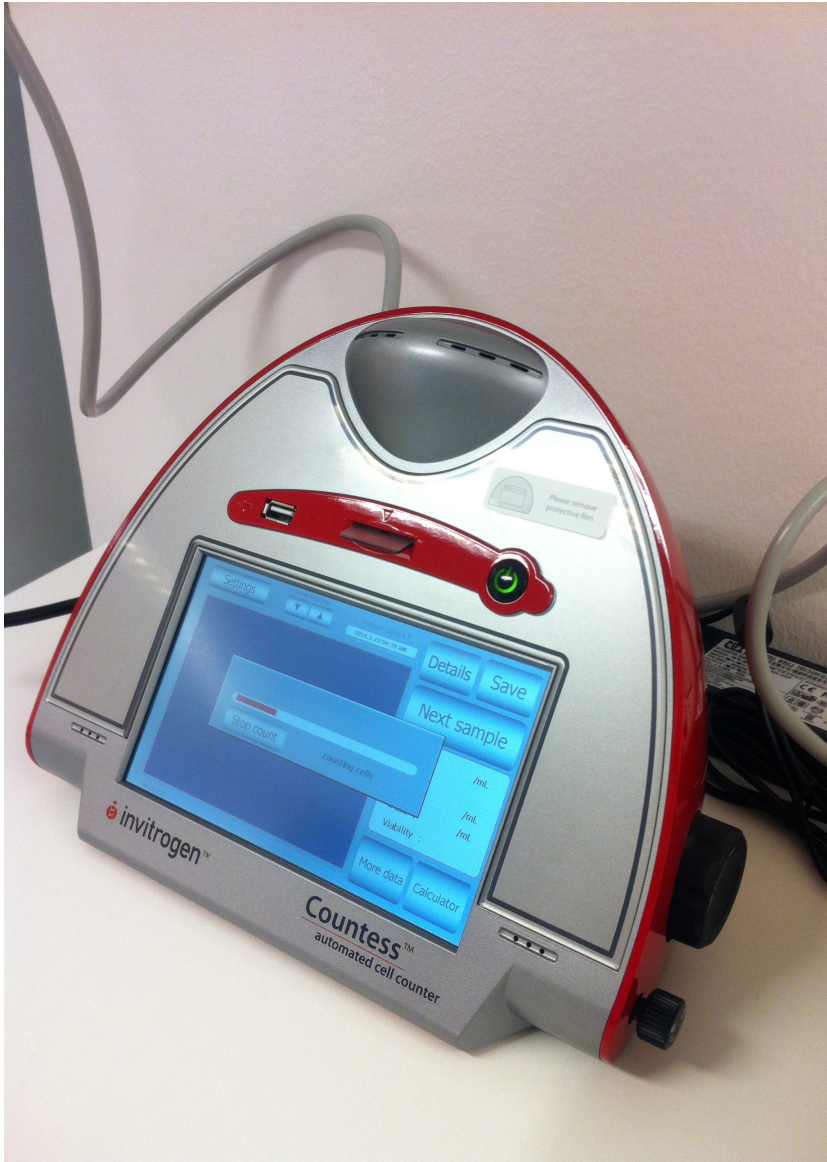
Figure 8: The Countess is a biotechnical oracle predicting that there are enough viable cells to transplant.
