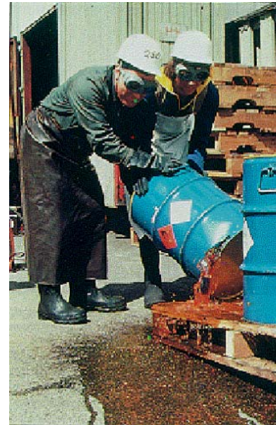
Figure 3.8: Drum ruptured by forklift (IMO, 1992)
