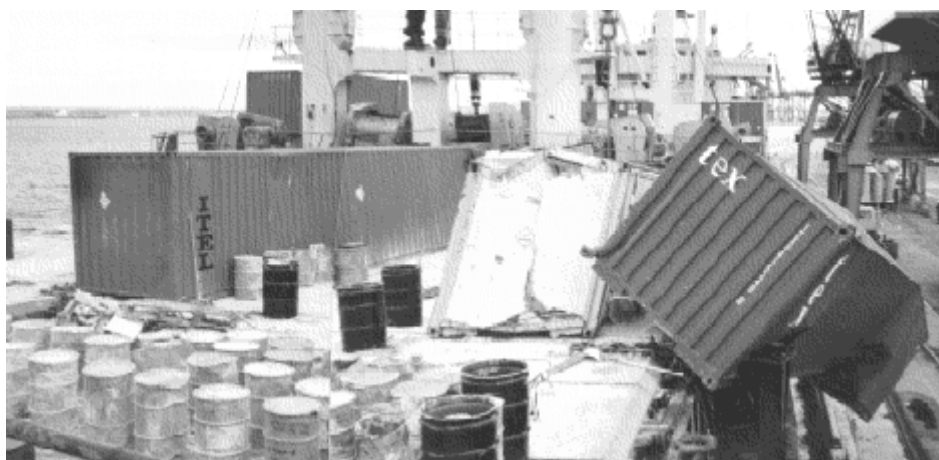
Figure 2.16: Damaged container on the no. 2 hatch cover of the m/v SCI on arrival in Port Baltimore (U.S. DOT, 1992)
