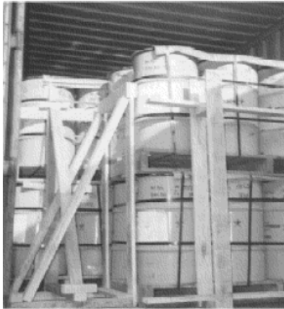
Figure 3.45: Palletised arsenic trioxide drums packed inside a container aboard the m/v SCI (U.S. DOT, 1992)
