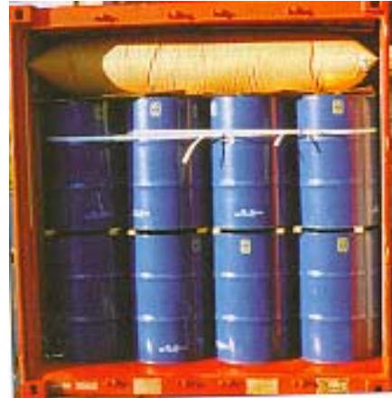
Figure 3.46: Un-palletised drums packed inside a container in accordance with regulations and good practices (Gefährliche Ladung, 1998)
