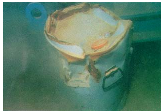
Figure 3.4: An impacted drum found on the sea floor by ROV (IMO, 1992)
