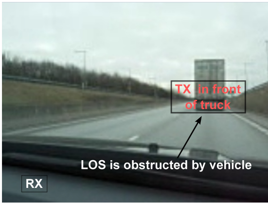
Fig. 1. Snapshot taken from the RX car, when the LOS was obstructed by a truck on a highway.
