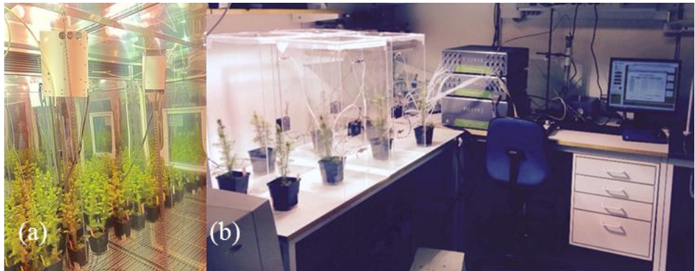
Figure 4. a) Seedlings were kept under controlled moisture, \text{CO}_2 concentration, and light intensity. b) ^{13}\text{C} pulse-labelling using plexiglass boxes connected to Picarro analyzer (Paper V).
