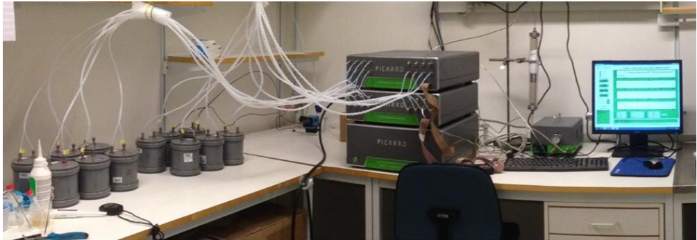
Figure 3. PVC microcosms containing soil were connected to Picarro analyzer (G2131-i) through PTFE tubes (Paper III).
