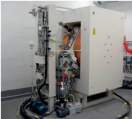
Fig 4.7: The GE PETtrace cyclotron in Lund.
