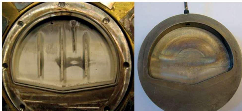
Fig 6.6: The old silver target (left picture) with support bars clearly suffers from silver colloid problems originating from the deterioration of the silver because of the proton beam power. The first Nb-body (right picture) was intact even after 8 months of daily productions
