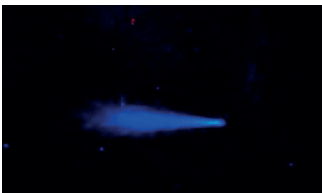
Fig 4.8: The GE PETtrace beam exiting the cyclotron into atmospheric air (range 25-30 cm) as monitored from the side, after passing 1.25 mm of Al.
