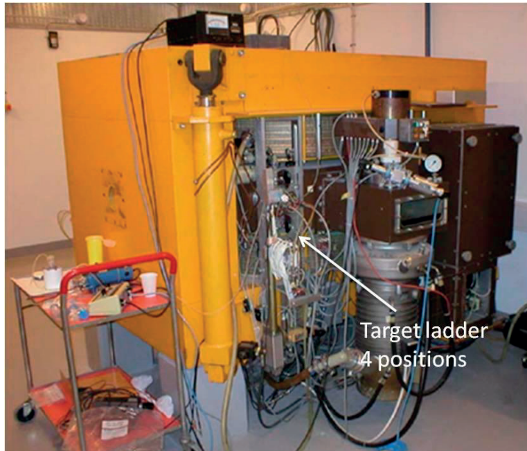
Fig 4.1: The Scanditronix MC 17 cyclotron installed inside the bunker in Lund. The MC 17 machine is equipped with a target ladder that can hold 4 different targets.
