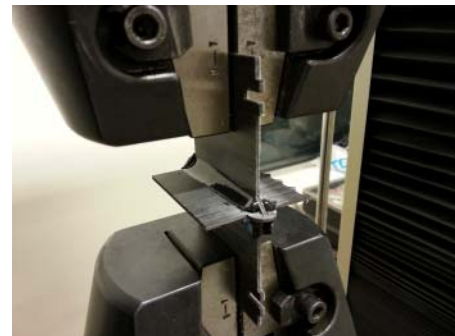
Figure 7. Specimens attached to the tensile machine.
