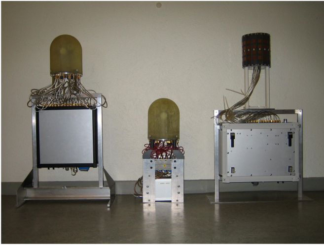
Fig. 3. Picture of the antenna structures and switches. (left) LU TX switch together and TKK semi-spherical antenna structure, (middle) TKK RX switch and TKK semi-spherical antenna structure and (right) the LU RX switch and LU cylindrical antenna structure.
