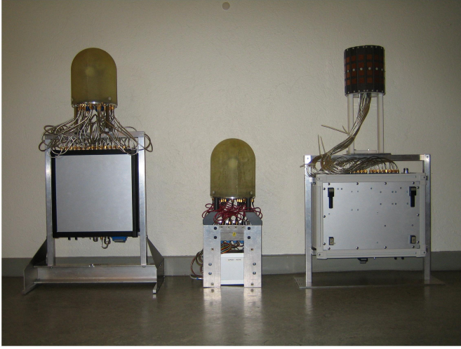
Fig. 3. Picture of the antenna structures and switches. (left) LU TX switch together and TKK semi-spherical antenna structure, (middle) TKK RX switch and TKK semi-spherical antenna structure and (right) the LU RX switch and LU cylindrical antenna structure.
