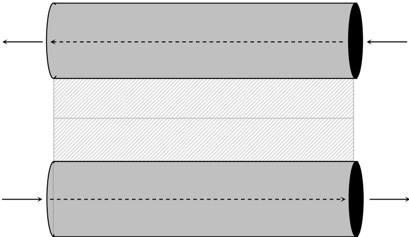
Fig. 5. A heat-exchanger control volume including two channels with 2 inlets and 2 outlets (solid arrows). The thermal interface (metal) is illustrated by the diagonally striped area, and the transport delays are illustrated by long dashed arrows.
