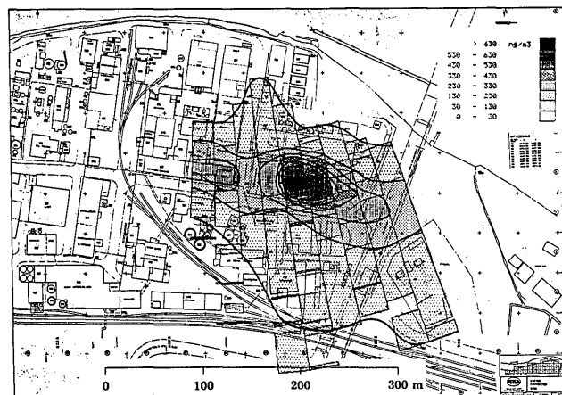
Fig. 8. Horizontal scan of Hg distribution over a chlorine-alkali plant.
