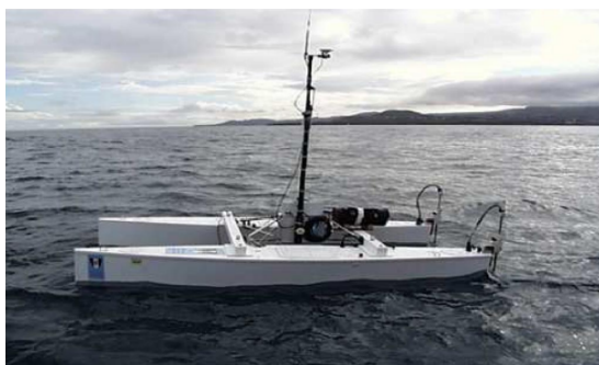
Figure 5: Delfim is an USV developed at ISR/IST to support gathering of data from a submerged craft [25].
