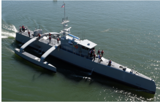
Figure 11: A prototype USV developed by DARPA in the USA, to hunt for submarines during month-long missions [30].
