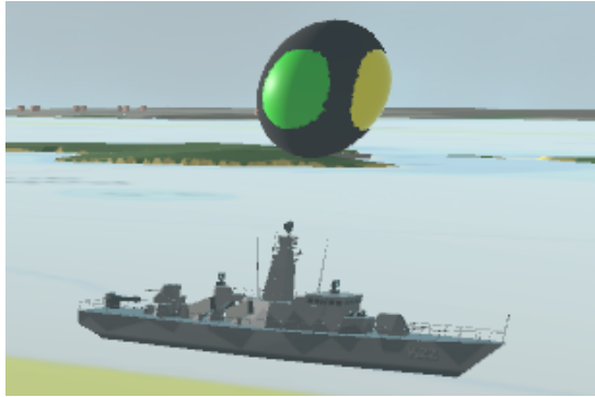
Figure 45: From the AIS data, the ship type, position and heading is extracted. From the ship type, a suitable 3D-model is chosen. The sphere is positioned above the position, and is colored according to the heading.
