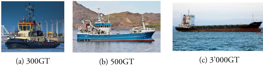
Figure 1: GT is a measurement unit of volume, and 260GTs is equal to about 1'000m^3 [5]. As a size comparison, a tug with around 300GT is seen in (a). (b) presents a fishing vessel with about 500GT, and (c) presents a container ship with about 3'000GT.
