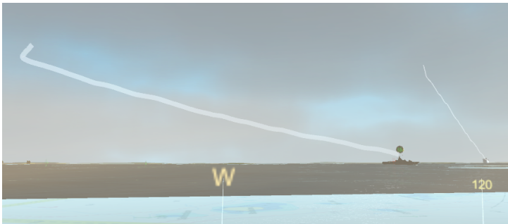
Figure 46: The bright bearing-lines in the sky indicates that both visual ships are steering to the right. The ship to the right is farther away, which is visualized with the thinner line. The ship to the left is going at a constant speed but has made a turn approximately 25 seconds ago. 30 seconds of history is presented in the CEP.
