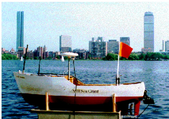
Figure 4: The USV Artemis, developed by MIT in 1993 [23].
