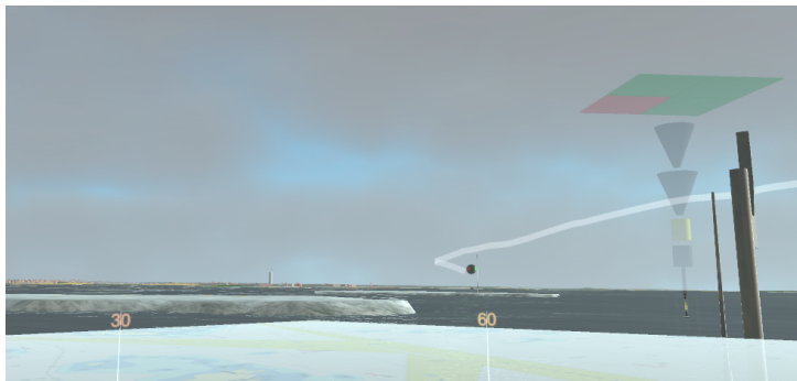
Figure 44: The South Cardinal Mark marks the grounding north from the Cardinal Mark (to the left in the image). The grounding is also marked with an iceberg.
