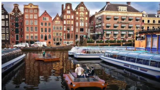
Figure 6: The Roboat is a small USV developed for shipping small sized goods and people through the canals in Amsterdam [26].
