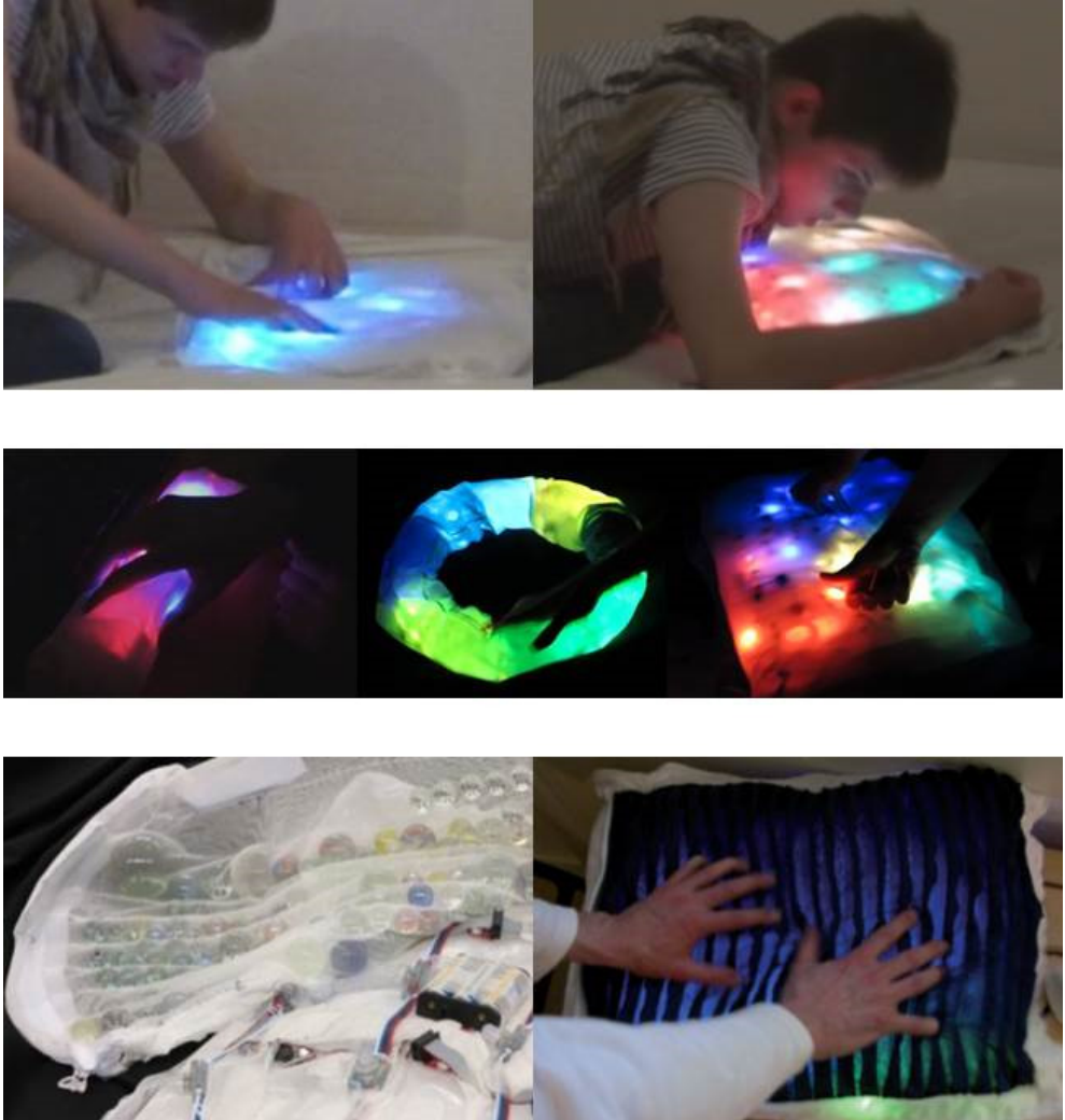
Figure 3.3. MalleablePillow . Top row: Co-located and gradual coupling. Middle row: Different physical shapes. Bottom row: Electronics/padding and black side of cover.
