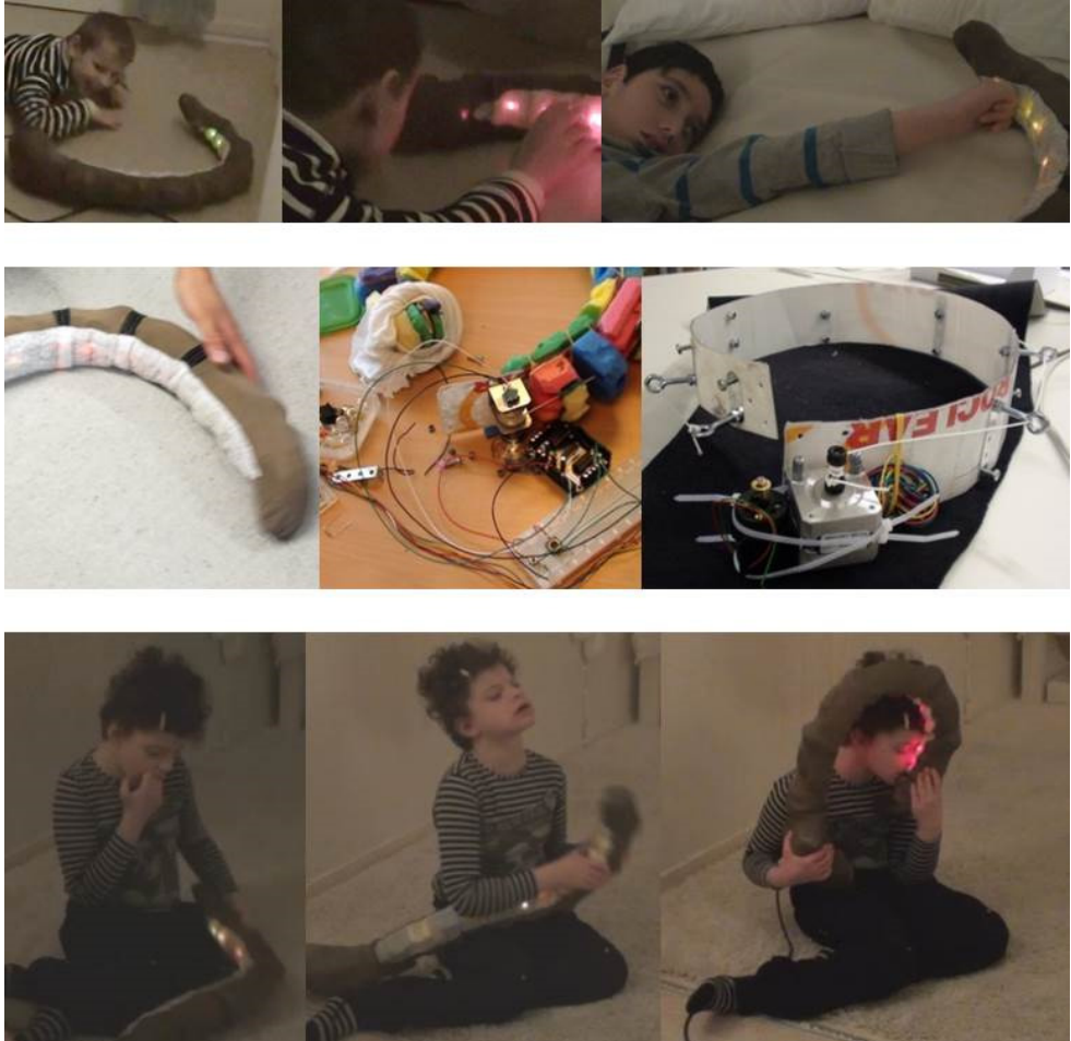
Figure 3.8. LivelyForm . Top row: Light and shape changing (left), reacting to ‘aura’ (right). Middle row: Construction; capacitive zones in the fabric (left), foam body, Arduino board, encoder (middle). Springy plastic and motor (right). Bottom row: Movement invites movement.
