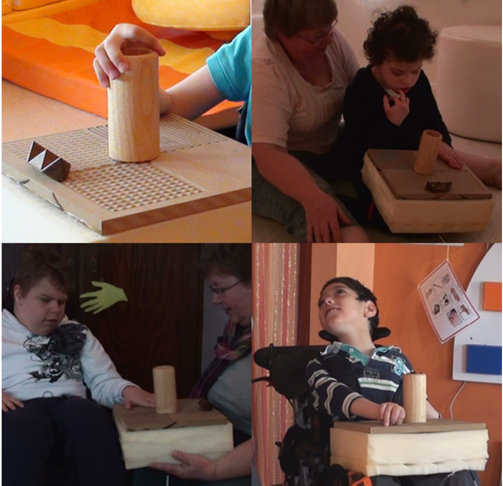
Figure 3.6. VibeBoard . Top row: Any wooden part vibrates. Bottom row: The vibration correlates with the stroking of the rifled parts.
