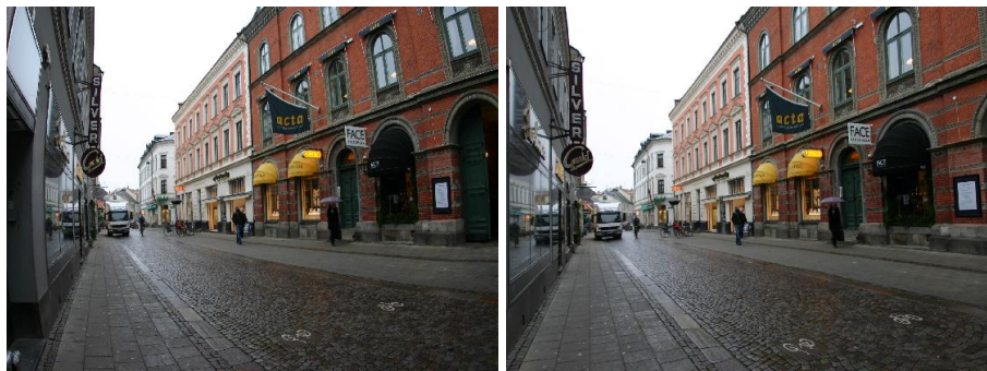
Figure 10.1: Left: An image taken with a fisheye lens. Right: The same image rectified when kernel voting is used to determine the radial distortion
