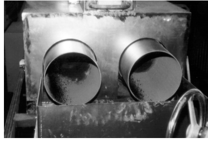
Figure 5.3: The drum granulator previously used to granulate the ETEC-dolomite, ash and water in Kalmar (Svantesson, 2000).
