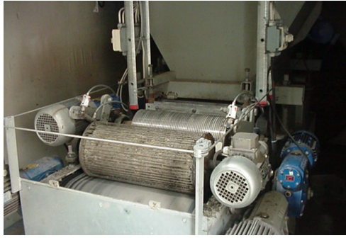
Figure 5.4: The roll pelletizer prototype, VAP-500, presented in Windelhed (2000).
