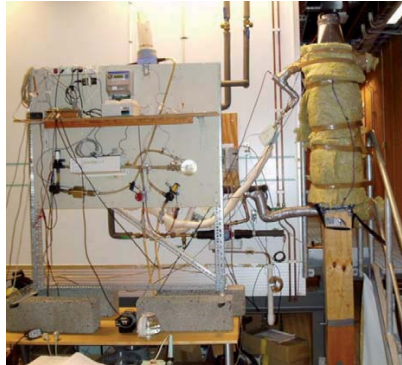
Figure 5. The heating rack is shown to the left and the insulated heat exchanger is shown to the right.
