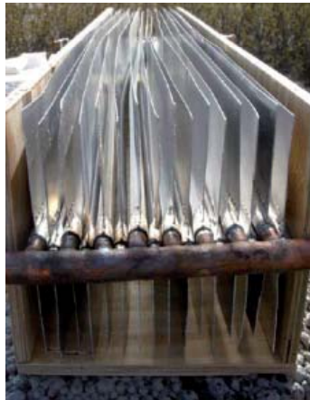
Figure 10. The heat exchanger. The fin pipes are not straight, resulting in a wavy path for the air through the exchanger.
