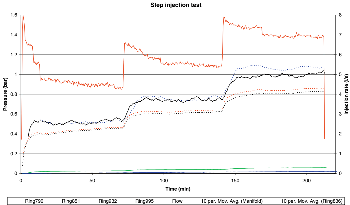
Fig. 5. Pressure increase and injection rate measured during the step injection test.
