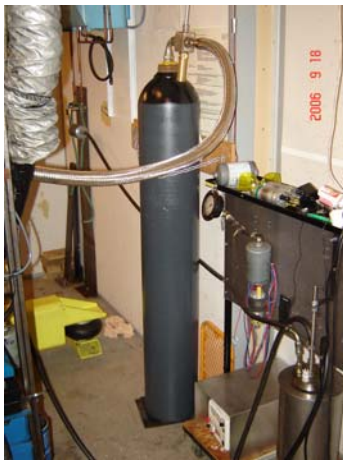
Figure 4 The pressure tank connected to the cylinder head by metal tubing.
