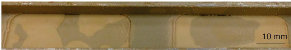
Figure 14 Image showing how the UHT fouling layer detaches from the metal surface during disassembly of the fouling unit when the geometry of the fouling coupon is not optimized.
