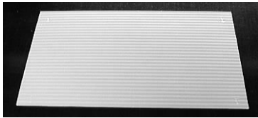
Figure 1.3. Example of a panel from a leveling test. In this test the surface should be as smooth as possible.
