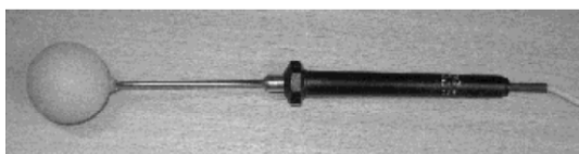
Fig 2. Globe thermometer consisting of a grey 38 mm acrylic ping pong ball around a Pt100 temperature probe [16]
