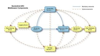
Figure 1: An overview of the ARC architecture showing the different components of the middleware.
