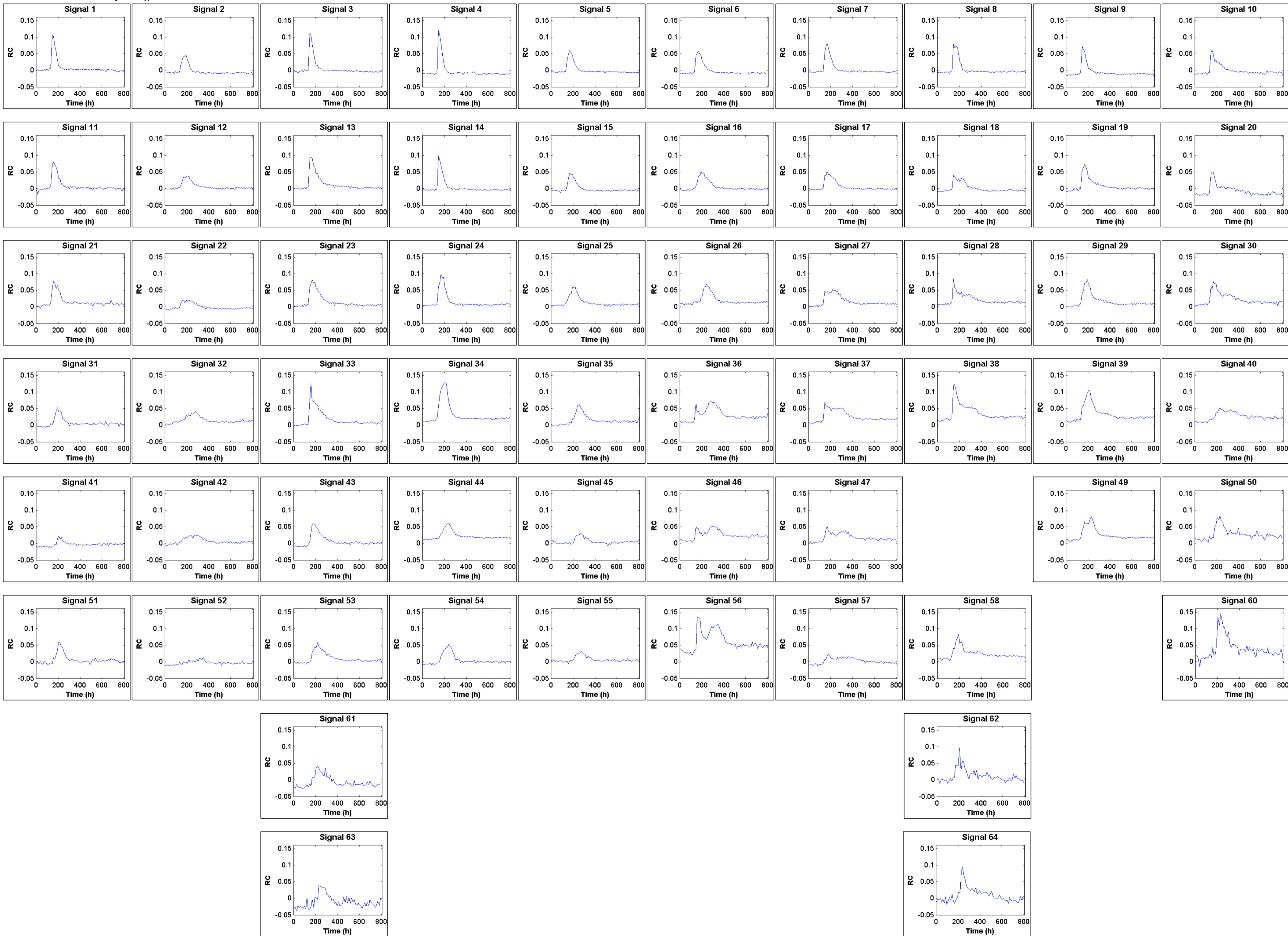
Figure 5. Schematic presentation of solute transport signals placed at the location of their corresponding measurement probes.
