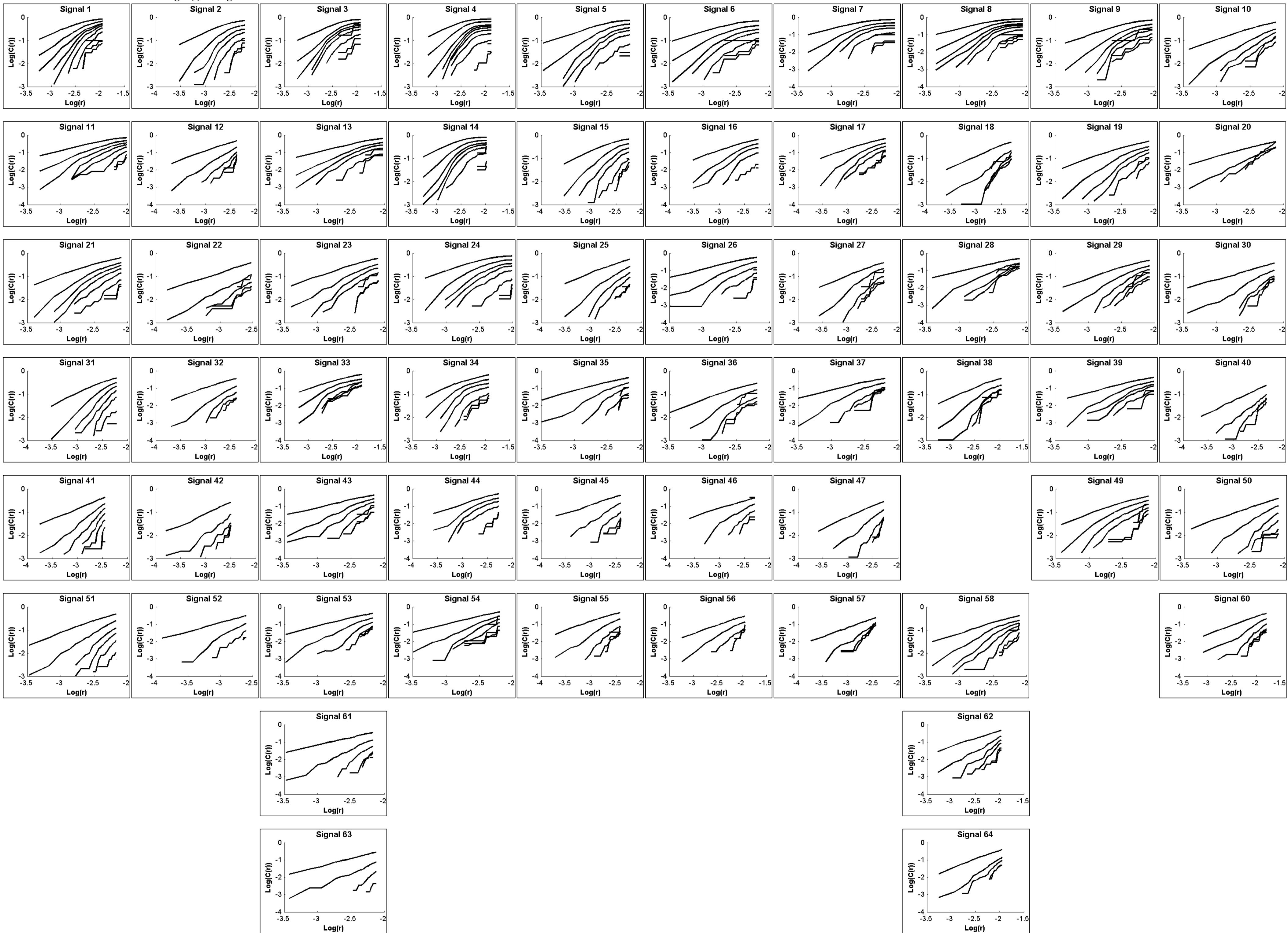
Figure 8. Schematic presentation of the plot of \log C(r) vs. \log r for solute transport signals placed at the location of their corresponding measurement probes.
