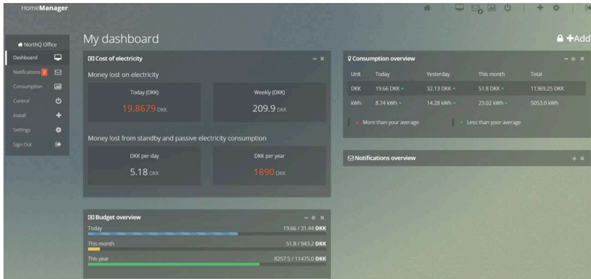
Figure 1 – Snapshot of consumption information available to SM customers online. ©NorthQ (used with permission) ( www.northq.com ).
