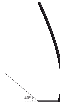
Figure 15. Proposed wall concentrator design, Wall prototype 6. The parabolic reflector has its optical axis tilted 40° from the horizontal and the solar cells are horizontal.
