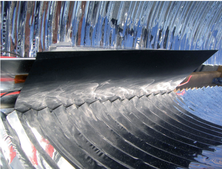
Figure 14.7 Non uniform irradiance distribution along the absorber created by the relatively large prisms.
