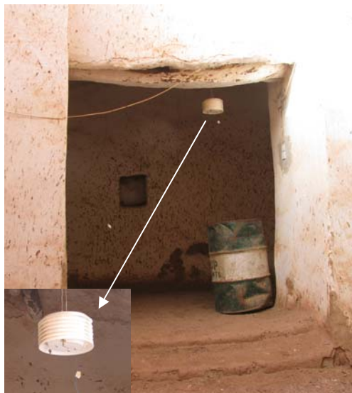
Figure 5.5 Outdoor temperature measuring loggers in Balat.
