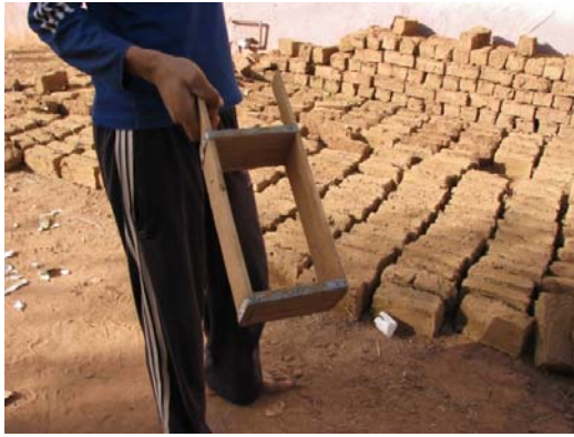
Figure 2.17 Moulds used in mud brick casting in the Dakhla oasis.
