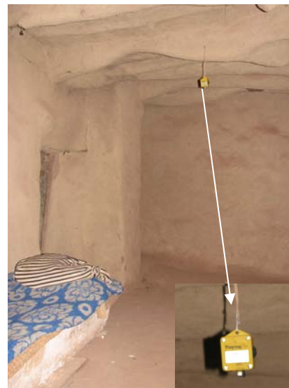
Figure 5.6 Indoor temperature measuring loggers in Balat.
