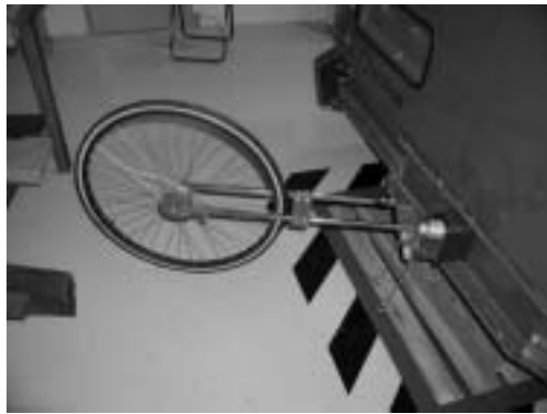
Figure A.8: The speed sensor, the fifth wheel.
