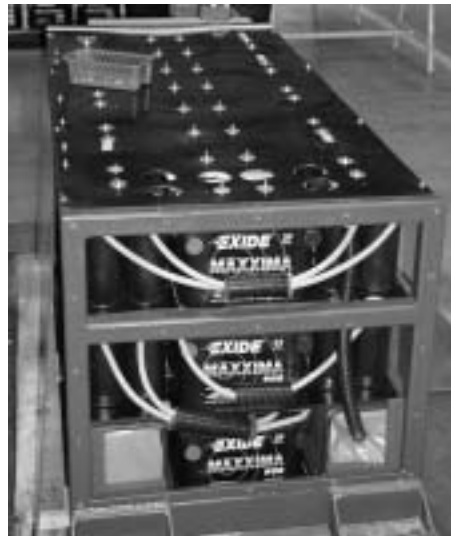
Figure 13: Driveline battery box with 44 units of 12 V batteries.
