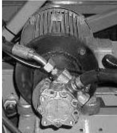
Figure 57: The servo pump and the electric motor.
