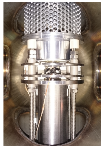
Figure 3.4. The ChristianTOF (top) and RamiTOF (bottom) spectrometers mounted on the vacuum chamber. Light enters from the left side and the sample is injected from below. A diode measuring the light flux is mounted downstream the chamber.
