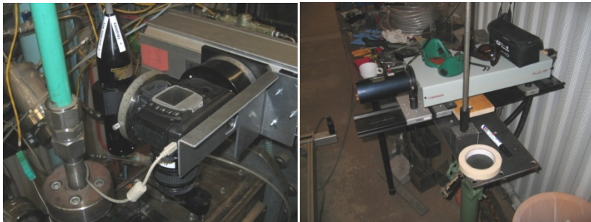
Figure 94: Closeup of PDA transmitting optics and Nikon D70s DSLR (left) and illumination laser for still photography (right)
