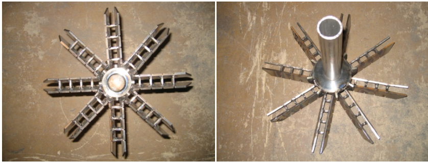
Figure 27: Flame holder seen from downstream (left) and upstream (right)
