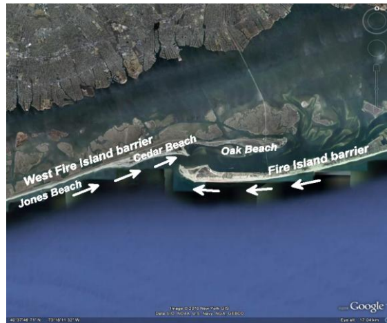
Fig. 5. Pathway of longshore sediment transport at the Fire Island inlet, New York, based on the description of Escoffier (1977) and Kraus et al. (2003) for a barrier overlap inlet.
