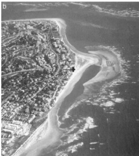
Fig. 8. Migration landward of attachment bar at Dewees Inlet (South Carolina) (Gaudio and Kana, 2001).
