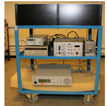
Figure 6.1. The mobile laser system used in the clinical trials. The black plates encase the breadboard system on the top shelf. Below are the temperature, piezo controller and water pump. The diode current supply is placed on the bottom on shock absorbing styrofoam.
