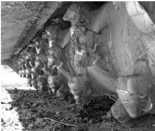
Figure 26. Crusher Roll with Teeth
