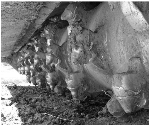
Figure 26. Crusher Roll with Teeth
