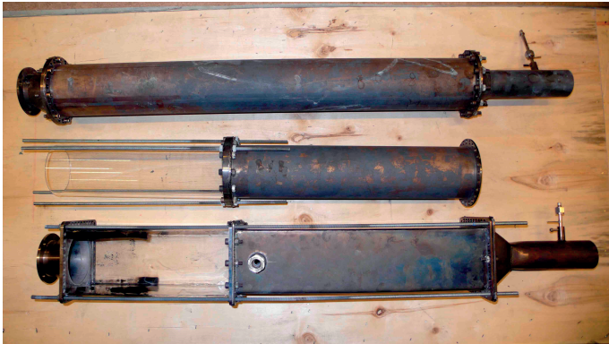
Figure 5.3: Three burner confinements used in atmospheric testing. Burner attaches from the left with quarl, which interfaces to the combustion liner. Liners terminate at right with a contraction and exhaust tube where the emission sampling port is located.
