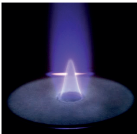
Figure 1: Photograph of a TMI seeded flame with \phi=1.0 using the central jet McKenna burner with laser induced fluorescence of Indium visible.
