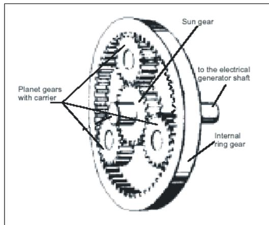
Figure 2-11: Planetary gear. The numbers of planet wheels are variable but influence the equations.
