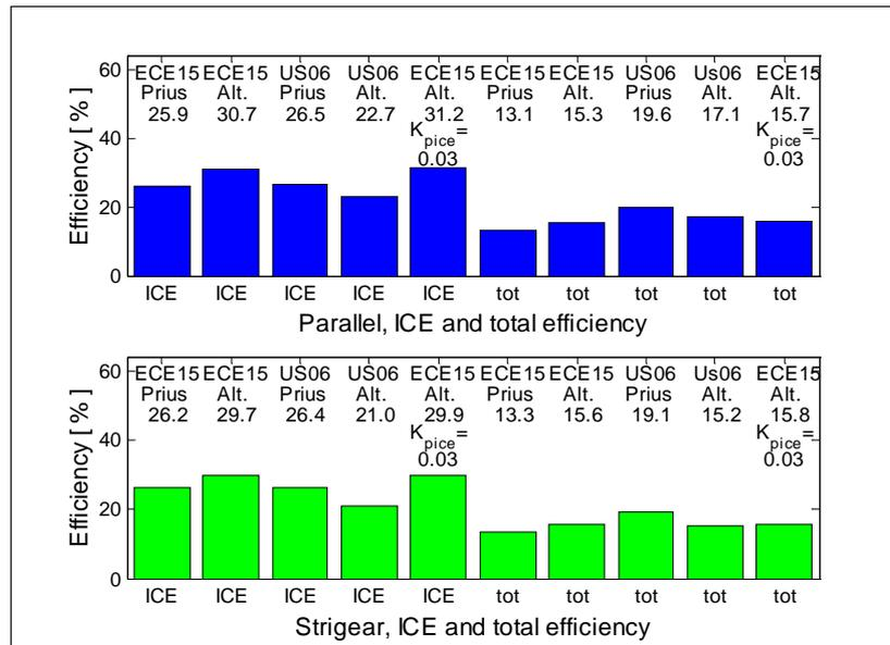
Figure 5-21: The graphs show the ICE- and the total efficiency. The efficiency values are corrected to correspond to  $SOC_{start} = SOC_{stop}$ . In the simulations the engine and motor sizes, driving cycle and charging gain have been varied.
