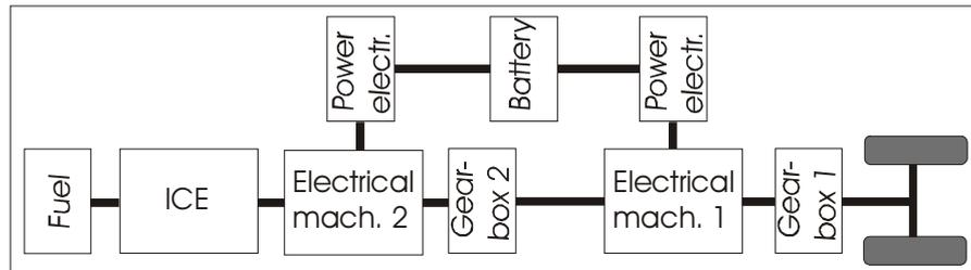
Figure 2-8: Parallel hybrid topology with one optional electric traction motor.
