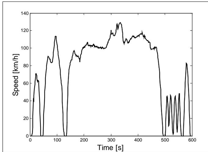
Figure 5-1: Drive cycle US06, velocity.
