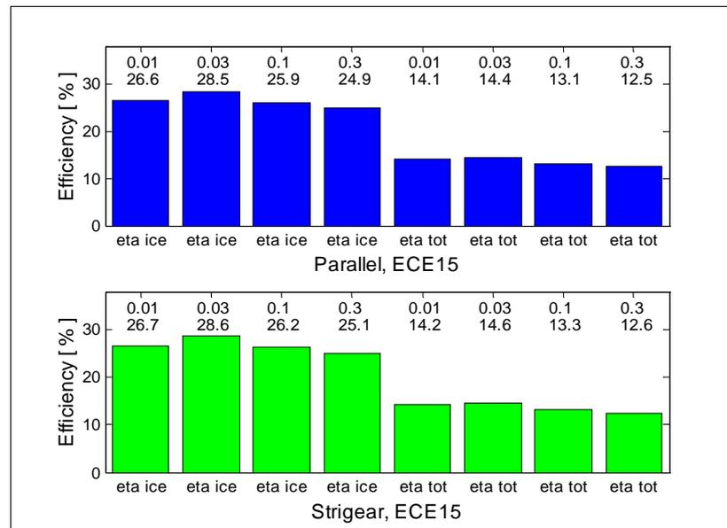
Figure 5-19: The figure shows the ICE- and the total efficiency for the vehicle simulated in ECE 15 and  $K_{pice}$  varied between 0.01, 0.03, 0.1 and 0.3. The efficiency values are corrected to correspond to  $SOC_{start} = SOC_{stop}$ .
