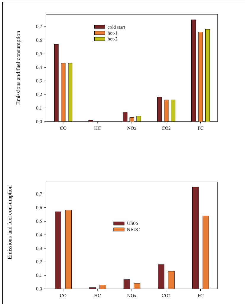
Figure 9-3: The figure shows the CO, HC and NO<sub>x</sub> and CO<sub>2</sub> emission (g/km) and the fuel consumption (FC) (l/10km). The upper graph shows the US06 cycle. The lower graph shows US06 cycle and a variant of ECE15, called NEDC and viewed in figure XX, cold started at 22°C.
