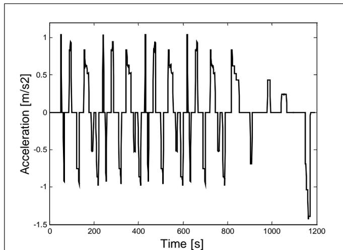
Figure 5-4: Drive cycle ECE 15, acceleration.
