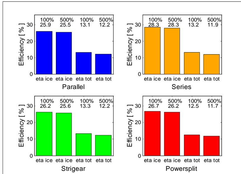
Figure 5-12: The graphs show the ICE- and the total efficiency for the vehicle, when simulated with  $R_{inner} = 100\%$  and  $500\%$  respectively. The efficiency values in the figure are corrected to correspond to  $SOC_{start} = SOC_{stop}$ .
