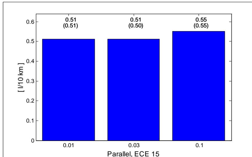
Figure 5-30: The parallel topology simulated with electrical machines of 1 kW and 65 kW. The “almost-one-electrical-machine-design” has been simulated with varied  $K_{pice}$  (0.01, 0.03 and 0.1). These results can be compared to the ones presented in Figure 5-15, the results of which are given in parenthesis in this figure.
