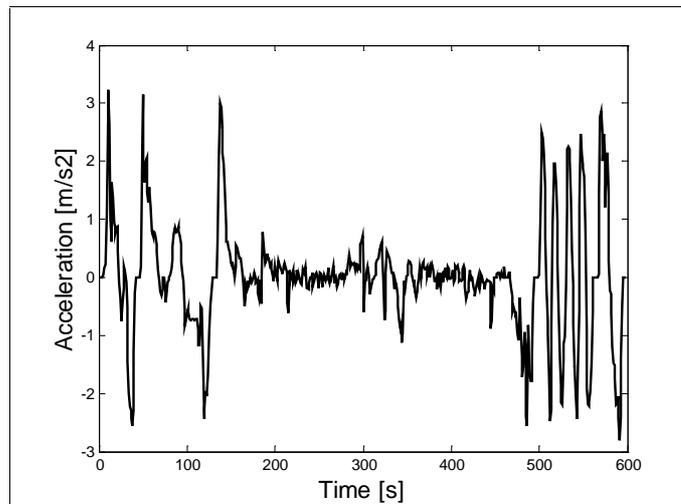
Figure 5-2: Drive cycle US06, acceleration.
