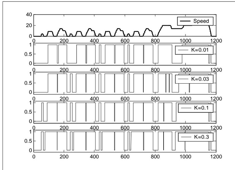
Figure 5-31: The graphs show different mode switching for strigear topology, depending on the chosen charging gain,  $K_{pice}$ . The uppermost graph shows the speed (m/s) for ECE 15. The other graphs show the strigear mode switching. 1 is equal to parallel mode and 0 is equal to series mode.
