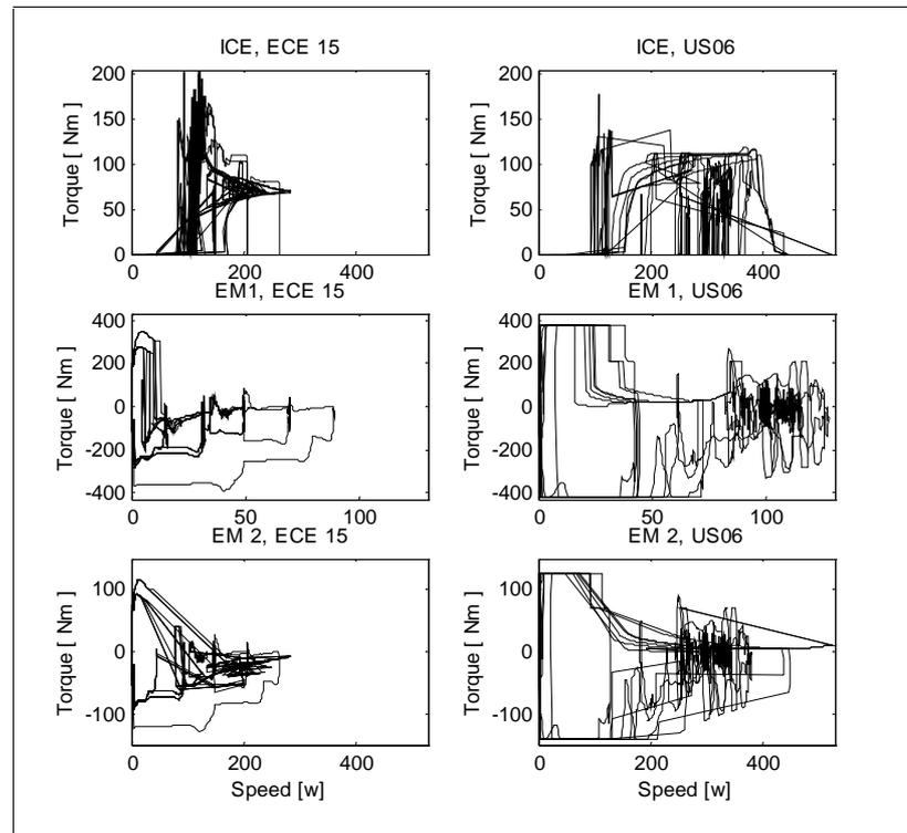
Figure 5-9: The graphs display speed vs torque for the parallel topology driving ECE 15 and US06, with  $\tau_{ICE} = 1$ . The graphs show, from top to bottom, ICE, electric motor 1 and electric motor 2.
