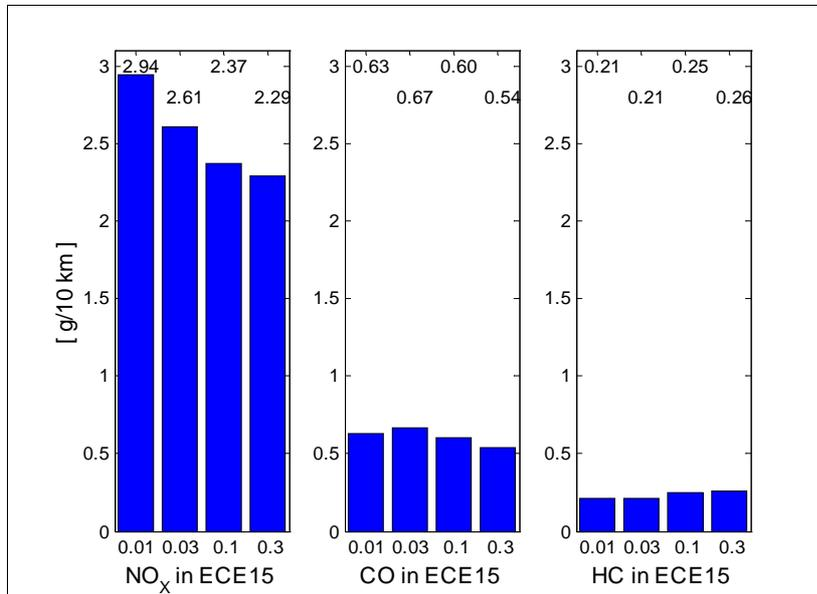
Figure 5-18: The graphs shows the emissions in g/10 km while driving the parallel topology in ECE 15 and varying  $K_{plce}$  between 0.01, 0.03, 0.1 and 0.3. The values are adjusted to correspond to  $SOC_{stop}$  equal to  $SOC_{start}$ .
