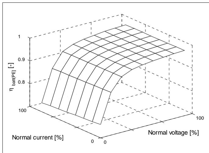
Figure 3-7: The normalized value for power converter efficiency.
