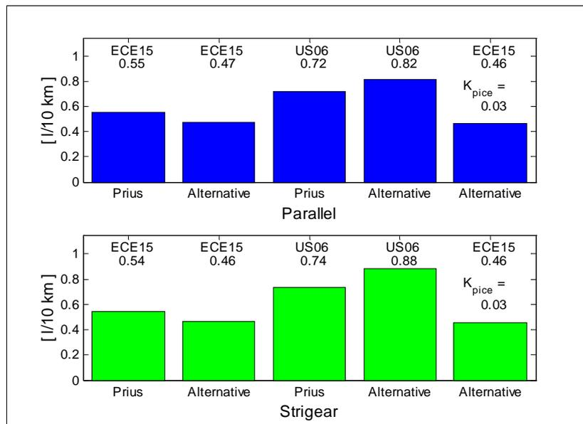
Figure 5-20: The figure shows the fuel consumption when simulating parallel and strigear topology, using different engine and motor sizes as well as varying the charging gain,  $K_{Pice}$  in the last simulation.
