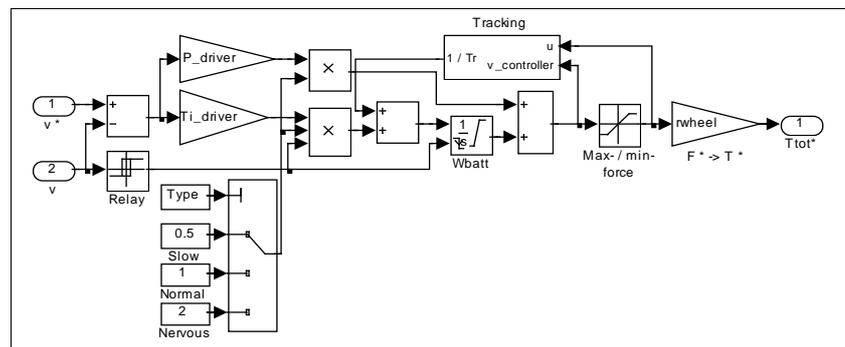
Figure 4-12: Inside the driver block consisting the PI-controller.
