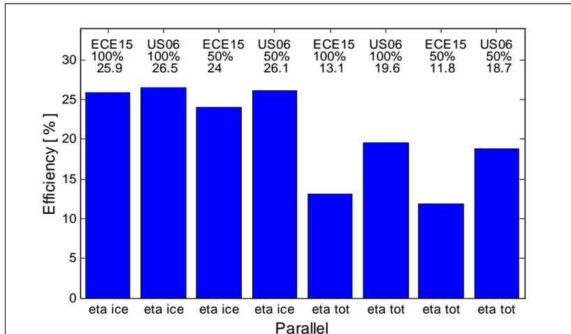
Figure 5-14: The figure shows the ICE- and the total efficiency for the vehicle, simulated with 100% and 50% battery, using both driving cycles. The efficiency values are corrected to correspond to  $SOC_{start} = SOC_{stop}$ .
