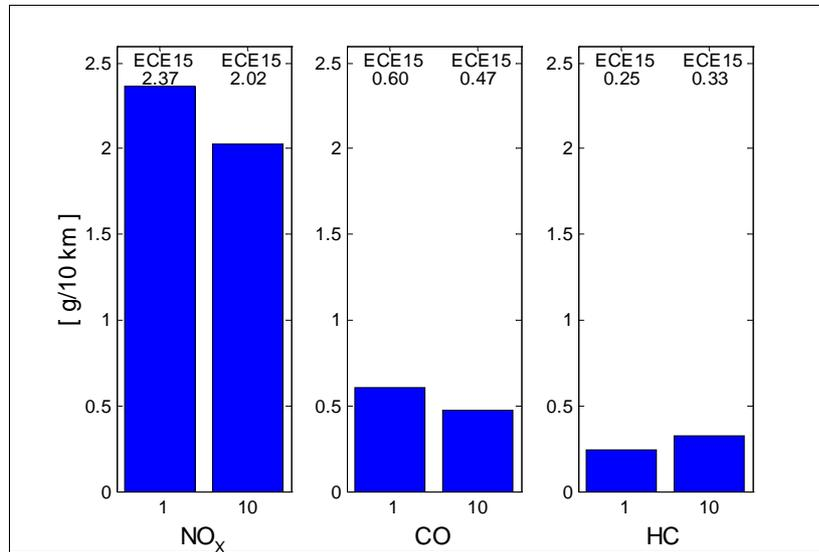
Figure 5-8: Emissions in g/10 km, while driving the parallel topology in ECE 15 and varying  $\tau_{ICE}$  1 and 10 seconds. The values are adjusted to correspond to  $SOC_{stop}$  equal to  $SOC_{start}$ .
