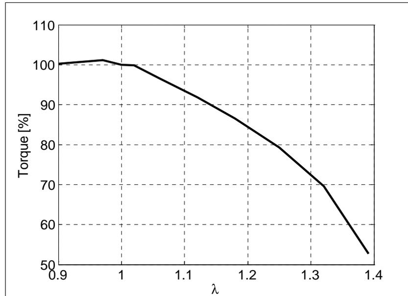
Figure 2-6: Torque reductions as function of  $\lambda$ .
