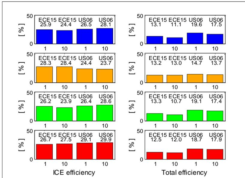
Figure 5-10: The graphs show the ICE- and the total efficiency for the four topologies. The efficiency values are corrected to correspond to  $SOC_{start} = SOC_{stop}$ . The graphs represent, from top to bottom; parallel-, series-, strigear- and power split topology.
