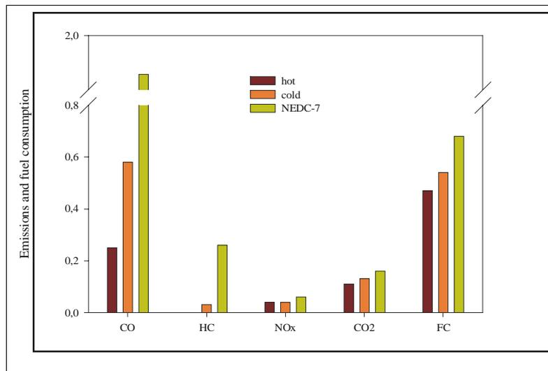
Figure 9-2: CO, HC, NO<sub>x</sub> and CO<sub>2</sub> emissions (g/km) and fuel consumption (l/10 km) in test-driving the variant of ECE15 viewed in figure XX. The tests shown have been hot and cold started at 22°C and cold started at -7°C (NEDC-7).
