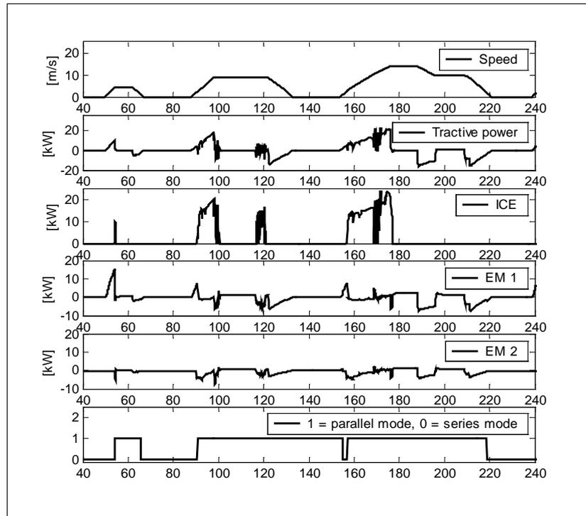
Figure 5-27: The figure shows the engine and motor power supply in the timeslot 40 - 240 seconds, when driving the *strigear* topology in ECE 15.
