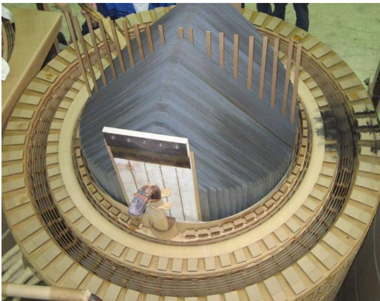
Figure 104: Serial auto-transformer winding internal fault in phase L2 was close to the 110kV connection point.
