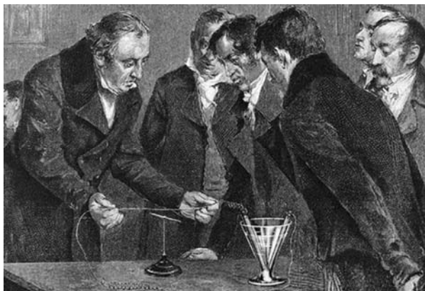
Fig. 2.1.1 Physics was “easy” in the 19 th century. The Danish physicist Hans Christian Ørsted accidentally discovered electromagnetism on his messy table as he short-circuited a Volta pile and noticed the reaction of a nearby compass needle.
