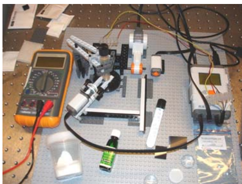
Fig. 4.4.5. Automated polarimetric goniometer made from inexpensive LEDs, film polarizers, LEGO and controlled by a LabView compatible Mindstorm micro-processor. The setup was assembled during an exercise on scattering from powdered milk during a workshop in Lima, Peru 346 .
