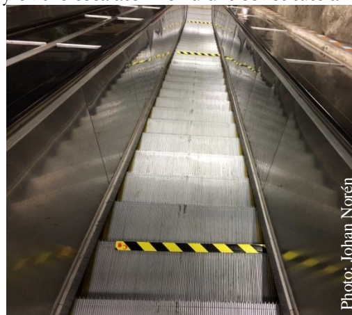
Figure 41. A picture of the segment marker (tape) in the escalator during the Västra Skogen experiment.
