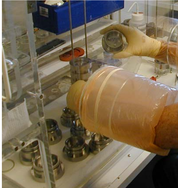
Figure 15. Unloading an SDI cascade impactor during AOE-01. The procedure needs to be carried out inside a glove box so as to prevent contamination.
