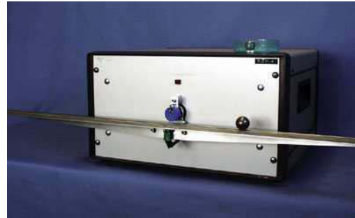
Figure 9 The ball and beam process.
