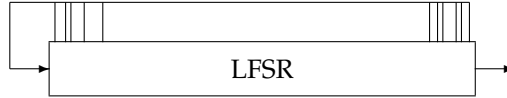
Figure 3.1: The characteristic polynomial a(x) = g_1(x) + x^M g_2(x) corresponds to an LFSR with taps concentrated to two groups.
