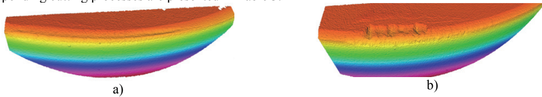
Fig.8 Comparison of tool wear for different tools when machining hardened high C-Si HCCI at v_c = 160 m/min: a) BCBN; b) HCBN
