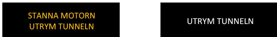
Figure 2. Examples of TIS with a two-line message in amber or a one-line message in white.
