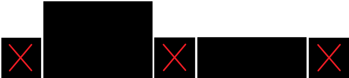
Figure 1. Schematic representation of the layout of information signs under consideration. The layout may include two panels of the same size (top) or a larger panel on the side of the emergency exit (bottom).
