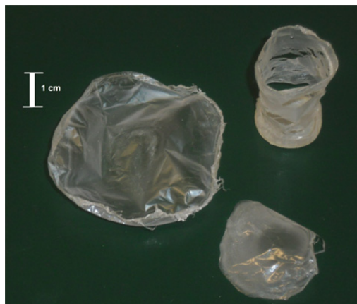
Figure 5.10 Poly(3-HP) produced from 3-HPA by recombinant E. coli BL21(DE3) expressing PduP and PhaC cs .
