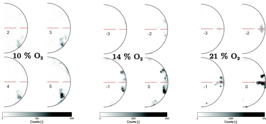
Figure 18 - Initial soot distribution for, from left to right; 10, 14, and 21% inlet  $O_2$  mole fraction. The numbers in each image indicate the crank angle degree after TDC, the dashed line indicates the jet axis.
