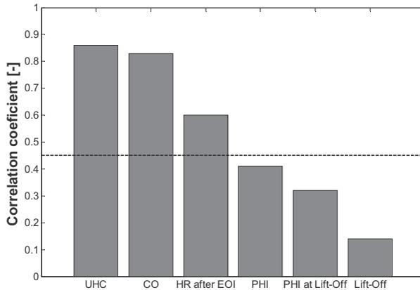
Figure 16 - Correlation coefficients between engine-out soot particle mass and different parameters. The UHC and CO emissions has the unit  $\text{g}/\text{kg}_{\text{fuel}}$ . The dashed line indicates the level that the correlation coefficient should exceed to be statistically significant, based on a one-tailed t-test with the confidence level of 95%.
