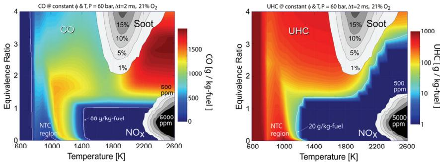
Figure 8 -  $\text{NO}_x$  and soot yield as function of equivalence ratio and temperature. The left figure is extended with the CO yield and the right figure is extended with the UHC yield. The yield is obtained from a homogeneous reactor simulation of an n-heptane/air mixture. The ambient pressure is 60 bar and the reaction time is 2.0 ms. [37]
