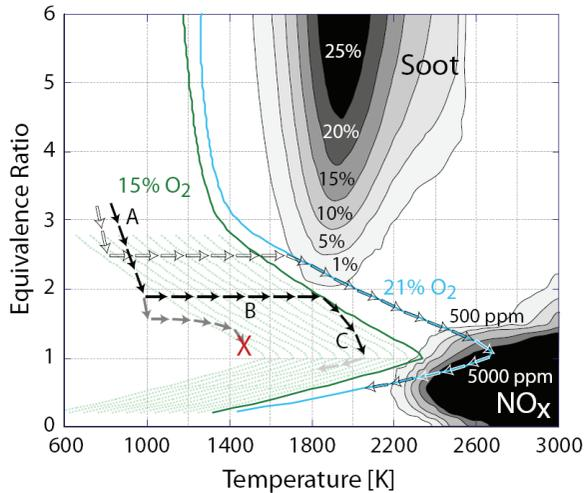
Figure 7 - Soot and  $\text{NO}_x$  production zones as function of temperature and equivalence ratio. The yield is obtained from a homogeneous reactor simulation of an n-heptane/air mixture during 2.0 ms. The adiabatic flame temperature is shown by the turquoise line at 21% ambient oxygen concentration, and the green line at 15% ambient oxygen concentration. [18]
