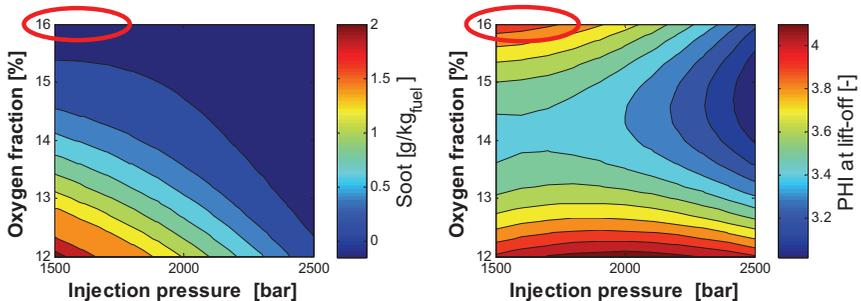
Figure 15 - Contour plot of  $\Phi$  at lift-off and engine-out soot emissions. The graphs show the combined effect of injection pressure and  $O_2$  mole fraction. The red oval indicates where the highest soot forming rate is expected.
