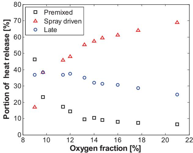
Figure 19 - Energy content in the premixed, spray-driven and late phase of the heat release rate as function of  $O_2$  mole fraction. The heat release is calculated using a volume trace according to Eq 28 and heat losses according to Eq:s 17, 18, and 19.
