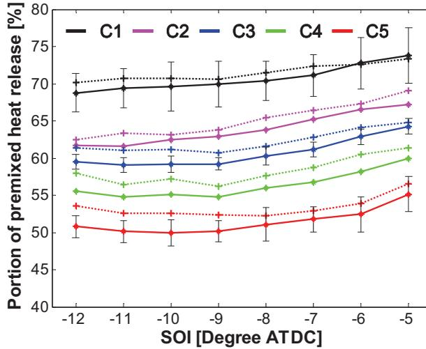
Figure 13 - Portion of heat release in the premixed combustion phase as a function of SOI for configuration 1 (C1) to C5 at 2.4 bar IMEP<sub>g</sub>. C1 is an all-metal engine and C2 to C5 are different set-ups of an optical engine. Higher configuration numbers are equal to more optical components. The deformations are considered for dashed curves but not for solid curves.
