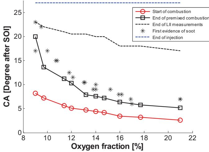
Figure 20 - Start of combustion, end of premixed combustion, time for the first soot appearance, and end of injection as function of inlet  $O_2$  mole fraction. All values expressed as CAD after SOI. The heat release is calculated using a volume trace according to Eq 28 and heat losses according to Eqs 17, 18, and 19.
