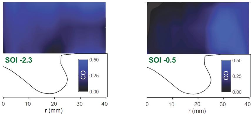
Figure 27 - Distribution of CO 50 CAD ATDC for the baseline load 3 bar IMEP<sub>g</sub>. The O<sub>2</sub> mole fraction is 15% and the start of injection timing in CAD ATDC is indicated in the images.
