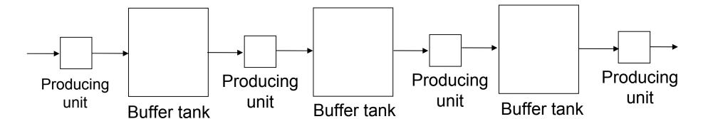
Furthermore, the topology of the production line could be more complicated, possibly containing recycle flows from one buffer tank to another, which will affect the optimal solution to the buffer management problem.
