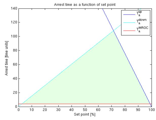
All combinations of arrest time and set point that are located within the triangle in the figure are allowed. The best choice of combination of set point and arrest time depends on the probability of larger disturbances than specified versus the effect on downstream processes when having rapid changes of the control signal.
